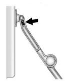
3. Release the prop rod from the inside cover by sliding the red clip down.
